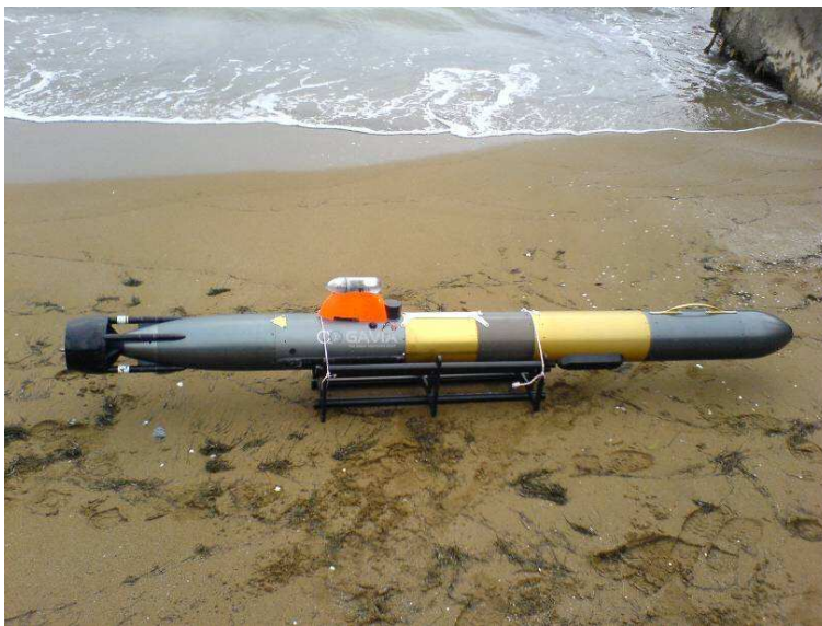
Figure 1: The Gavia AUV, total length 2.6m with the modules proposed here (counting from the right): Nose cone, battery module, GeoSwath, DVL, INS, control unit with tower, propolsion module.
