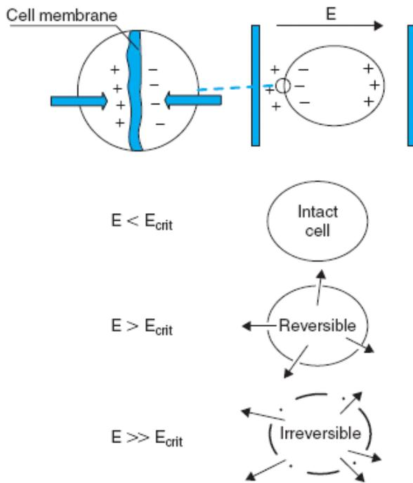
**Figure 1.** Schematic depiction of mechanism of membrane permeabilization by electrocompressive forces induced by an external electric field. Increasing treatment intensity will lead to formation of large irreversible membrane pores.  $E$  = Electric field strength,  $E_{crit}$  = Critical electric field strength [2].
