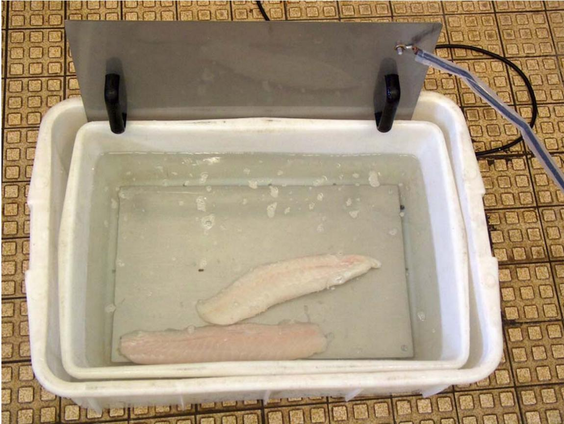
**Figure 3.** Samples of cod in container between two parallel stainless electrodes
