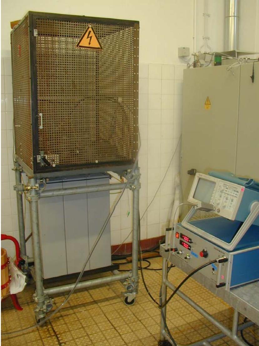
**Figure 2.** A high voltage pulse modulator (TU Berlin)
